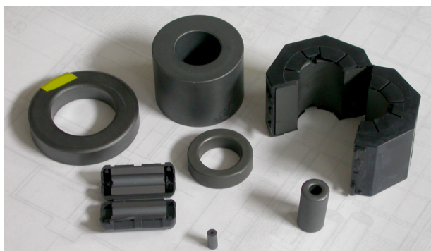
Fig 2 – Ferrites are made in many forms
